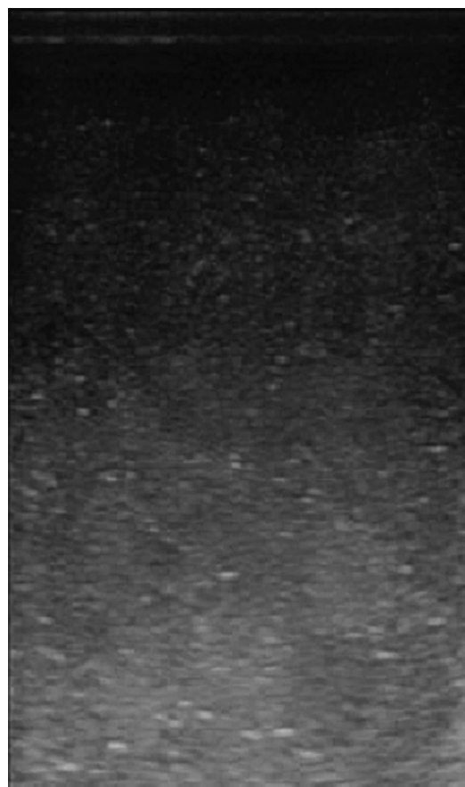
Figure 1 Gelatin phantom as seen by linear probe (12 tablespoons Jell-O, 4 tablespoons Metamucil).
