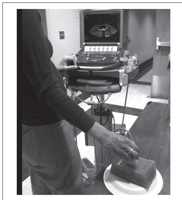
Figure 1. An operator imaging the gallbladder phantom with a phased array probe.
