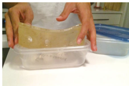
Figure 8. One side of the gel tilted out of the model's container in order to fill the lumens with liquid.
