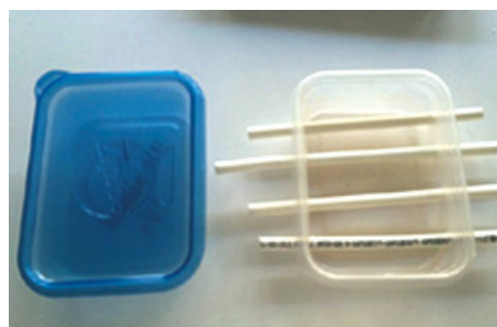
Figure 4. A plastic food storage container with plumbing tubing threaded through holes.
