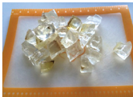
Figure 2. One-inch cubes of ballistic gel.
