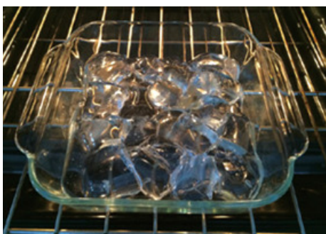
Figure 3. Melting ballistic gel in oven safe glassware.
