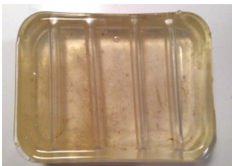
Figure 7. Gel model with four phantom lumens.
