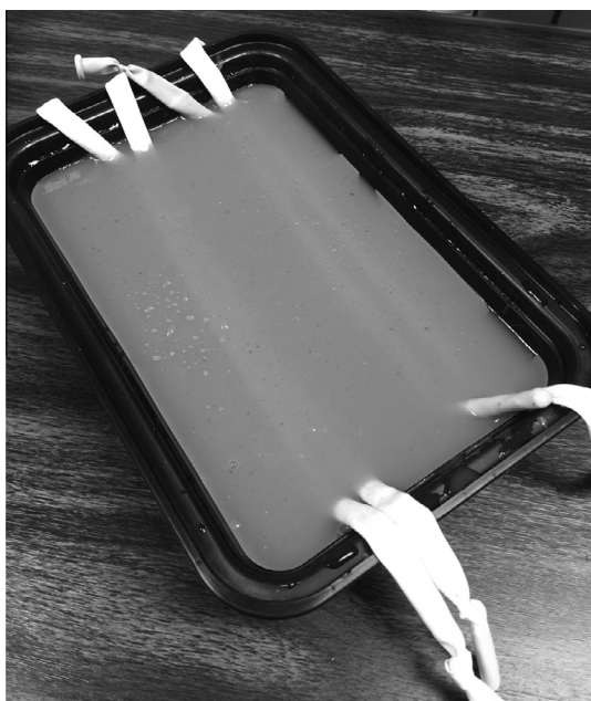
Figure 1 A completed 5% agar model with red dye in the matrix and two sets of vessel analogues.
