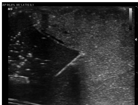
Figure 7. Needle tip and tracking within the abscess phantom. This image is after several aspiration attempts and demonstrates the absence of needle track artifacts with multiple uses.
