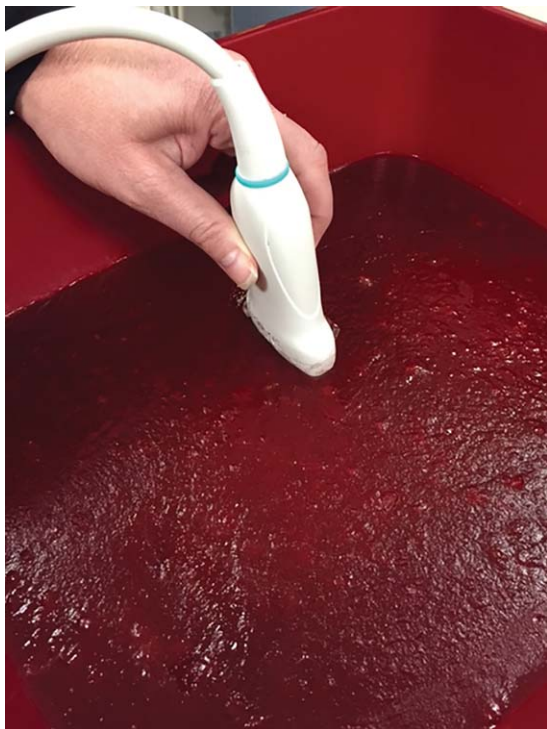
Figure 4. Ultrasound scanning of the phantom using a linear transducer. Notice the opacity of the phantom, which obscures the identification of the abscess by direct visualization.
