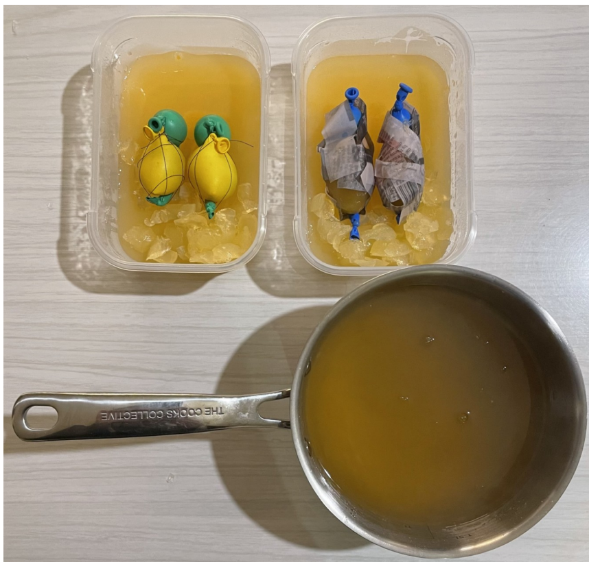
Figure 5: testes about to have the lower density agar poured around them
