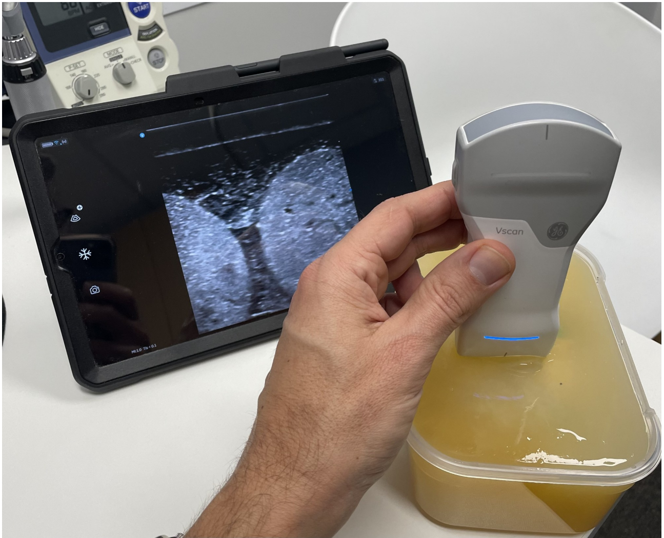
Figure 6: The finished phantom being scanned
